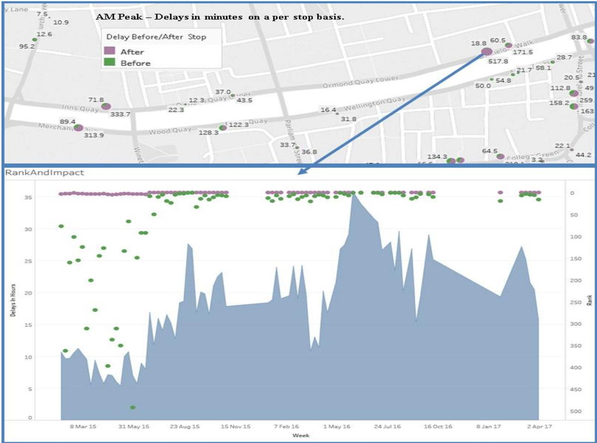
**Figure 11** Dual Axis Graph presents the Impact (delays in Hours) and ranking of bus stop with most delays
